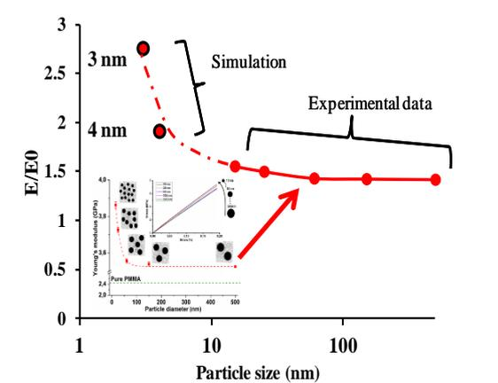
Figure 1: Experimental (elastic[1] and viscoelastic properties) and simulation[2] size effect evidence on elastic modulus of 4% silica-PMMA composites
